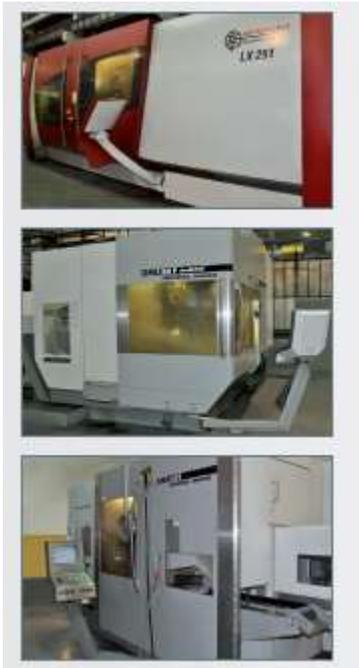
Team of CNC programmers utilises the great capabilities of CNC machine tools. Their tools of the trade include the following CAM systems: Master CAM, RCS and HyperMill. Plant operates a number of CNC machines of Swiss and German production. These include (among others): STARRAG LX 251, DMU 80P and DMP 60S.
